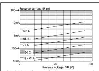
Fig.4. Typical reverse leakage current per diode;  $I_R = f(V_R)$ ; parameter  $T_j$
