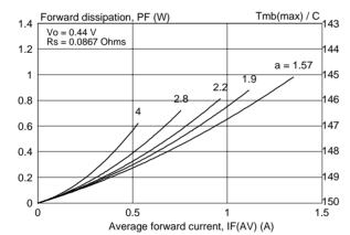
Fig.2. Maximum forward dissipation per diode  $P_F = f(I_{F(AV)})$ ; sinusoidal current waveform where a = f(AV).
