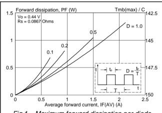
Fig.1. Maximum forward dissipation per diode  $P_F = f(I_{F(AV)})$ ; square current waveform where  $I_{F(AV)} = I_{F(RMS)} x \sqrt{D}$ .
